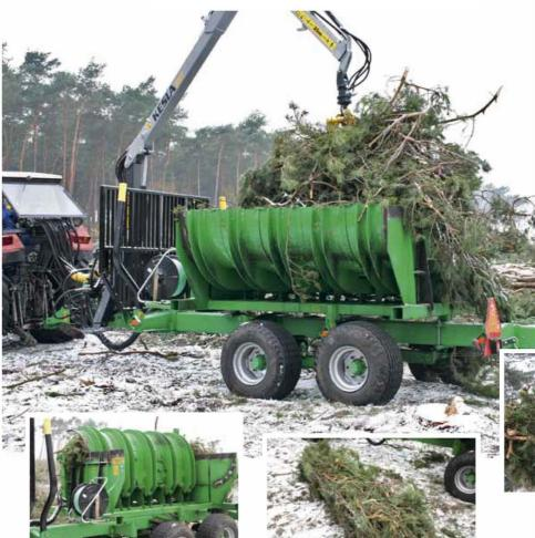
The Forest Biomass Baler for logging slash is mounted on a forest trailer. The device consists of 5 compressing sections mounted on a mutual mid-frame. Each section has a wall and moving elements powered by hydraulic cylinders which allows for compaction and strapping of the load. Strapping is carried manually using a PP tape and a strapping tool. The set has a hydraulic system with a hydraulic distributor steering the sections.
