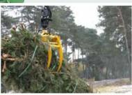
The system is powered from the hydraulic system of a tractor. The set is intended for mounting on the JAR-8 trailer equipped in a hydraulic crane, which in this case is used for loading logging slash and unloading strapped bales.
